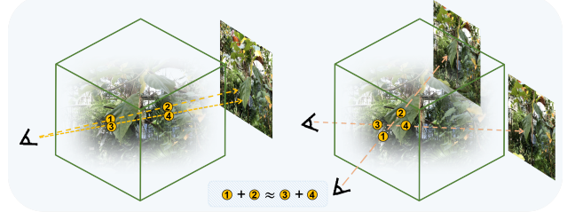
Figure 2. Illustrations of image structure (left) and cross-view consistency (right) from the perspective of volume rendering. For easy understanding, we placed images behind radiance fields (the cubes), and the two yellow circles on each ray denote the weighted colors sampled for volume rendering as Eq. (2). For each case, the volume rendering variance as Eq. (5) should be a small value.
