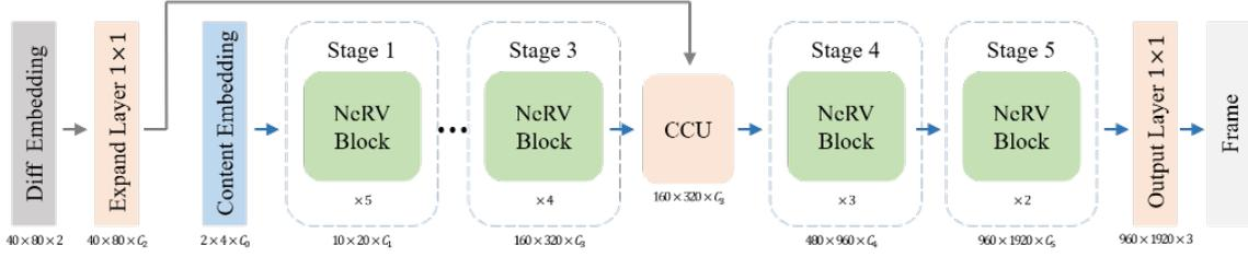
Figure 4. Architecture of decoder with CCU as fusion module for  $960 \times 1920$ .
