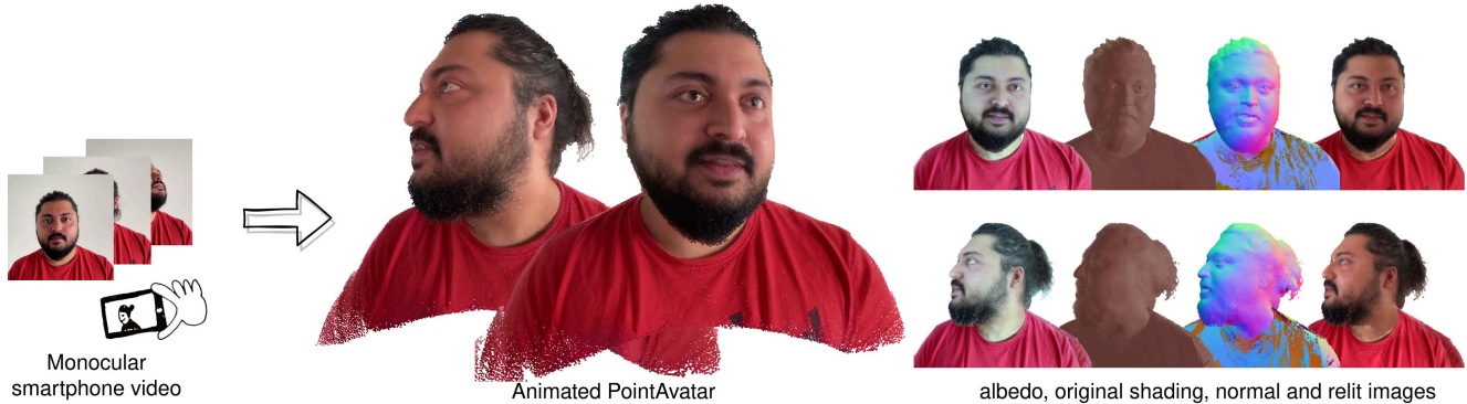
Figure 1. PointAvatar learns lighting-disentangled point-based head avatars from a monocular RGB video captured by a smartphone.
