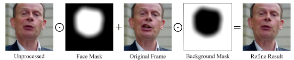
Figure 3. Post-processing for generated face pasted onto the original frame through a Gaussian-smoothed face mask.
