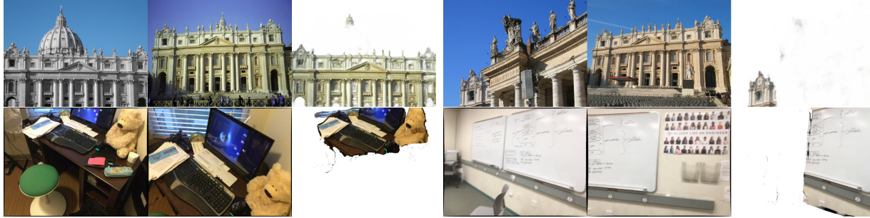
Figure 5. Visual Quality of the Reconstruction. We visualize 4 reconstructed images using estimated dense correspondences. In each group, from left to right is the source image, support image, and the reconstructed image. The areas of low confidence are filled with white color. In ScanNet where the confidence groundtruth is not available, we use forward-backward flow consistency mask as a replacement.
