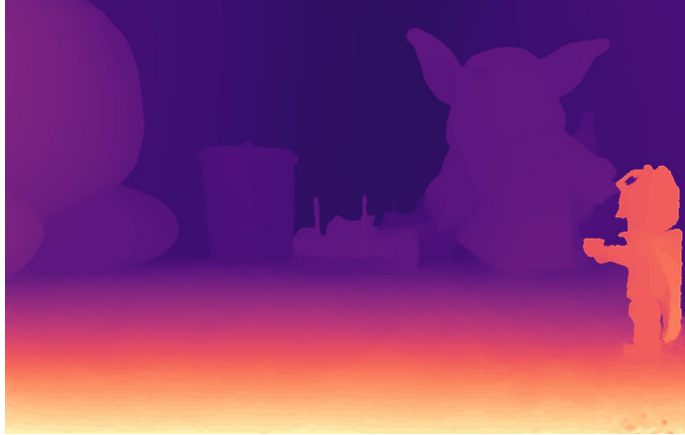
Figure 3. Disparity from iPhone. Using portrait mode, we obtained Dual-camera disparity using an iPhone 14 Pro.
