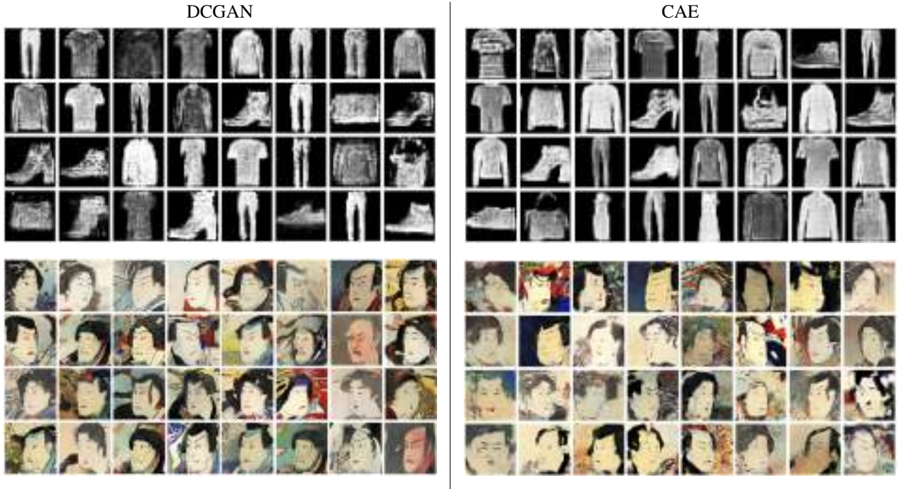
Figure 7. Images generated by Spider GAN on Fashion-MNIST and Ukiyo-E Faces, given the friendliest neighbor input as identified by SID. Both CAE and DCGAN result in images of comparable visual quality on Fashion-MNIST. However, for high-resolution image generation on 256-dimensional Ukiyo-E Faces, the fully convolutional structure of the CAE generator result in images of poorer visual quality than those generated by DCGAN.
