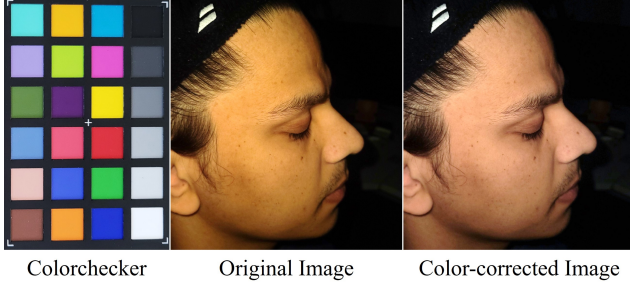
Figure 2. We found that the polarization filters introduce a color shift depending on the polarization direction. To this end, we perform a color calibration with a Macbeth colorchecker board which we capture in both scenarios (cross-, and parallel-polarized). We use an affine color correction to match both captures, and apply this transformation to recordings of all subjects.
