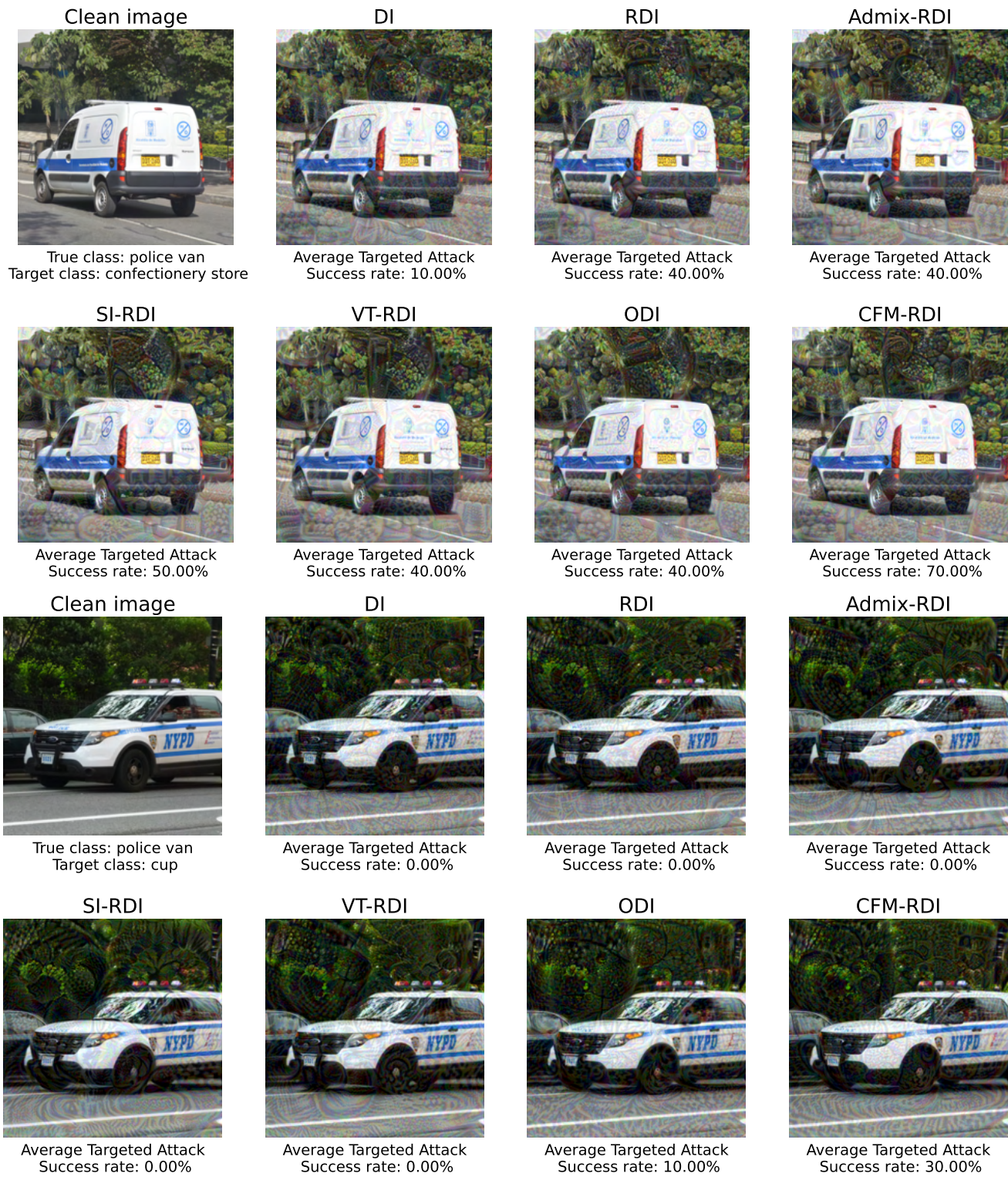
Figure 6. Visualization of generated adversarial examples. The source model is Inc-v3. Each average targeted attack success rate was calculated over the ten carefully selected target models, which are more difficult to confuse. For example, an average targeted attack success rate of 50% means that 5 out of 10 target models recognize the adversarial example as the target class.
