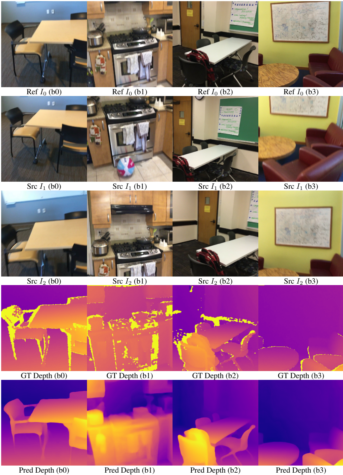
Figure 2. Training logs at last logging step on ScanNet [3] training set. Columns show samples and results of mini-batch ones b0, b1, b2, and b3. For the training logs, we show the color maps of the ground truth depths and predictions in the inverse space (i.e., disparity), so as to better align with the training loss calculated on the inverse depth domain.
