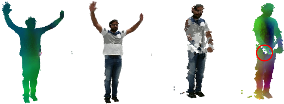
Figure S5. A qualitative result from real-scanned raw point clouds and the corresponding extracted features from DiffusionNet.
