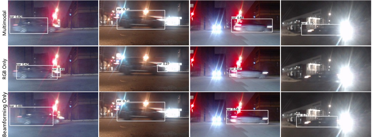
Figure 7. Additional object detection results on unseen scenes. We show the detections on unseen scenes with RGB-only, Beamforming-only and Multimodal methods. As can be seen, sound pressure signals via beamforming carry complementary information that results in superior detections for scenes where RGB images fail. Overall, multimodal detection method outperforms RGB-only and beamforming-only detections.
