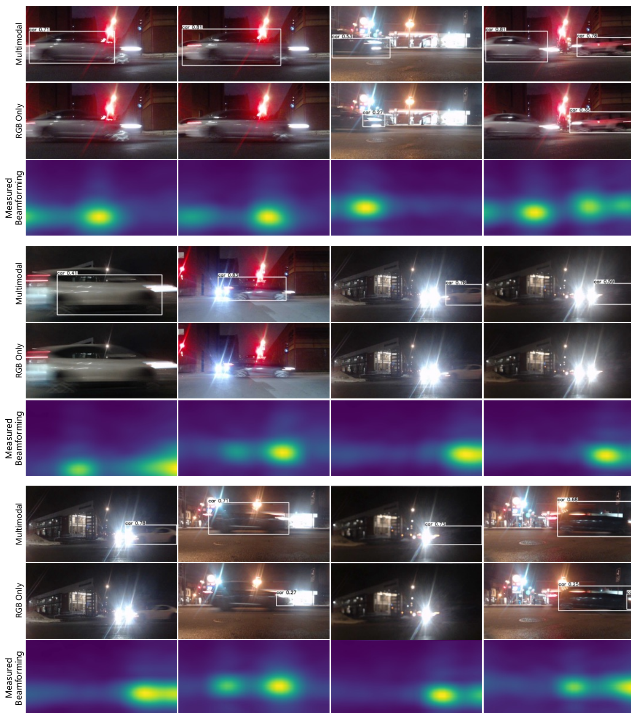
Figure 5. Additional object detection results on unseen scenes. We show the corresponding beamform maps (4000 Hz) for each RGB frame. The detrimental impact of glare and motion blur in low light conditions on RGB detection can be seen in the third row. Detection using beamforming maps circumvents these problems.
