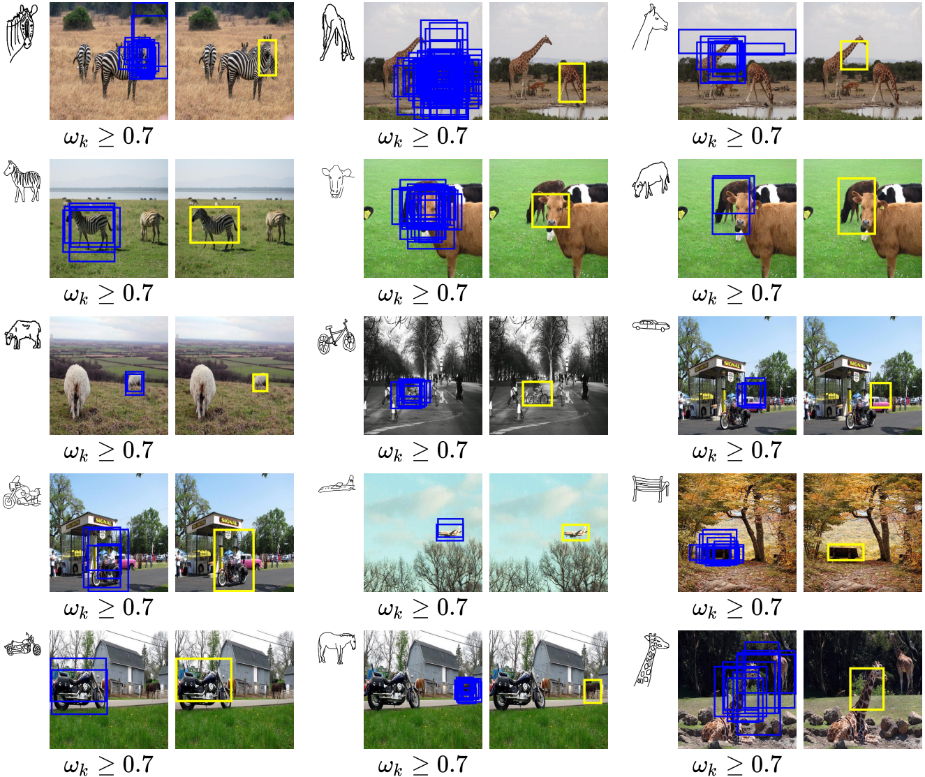
Figure A. Additional qualitative results for fine-grained and part-level object detection on SketchyCOCO. Note both the Blue and Yellow boxes are network predictions and not ground truth. The Blue boxes are predictions from the network prior to using Non-maximum suppression (NMS) with the confidence score of the predicted box \omega_k \geq 0.7 . The Yellow boxes are the resulting predictions after applying NMS with \text{IoU} \geq 0.3
