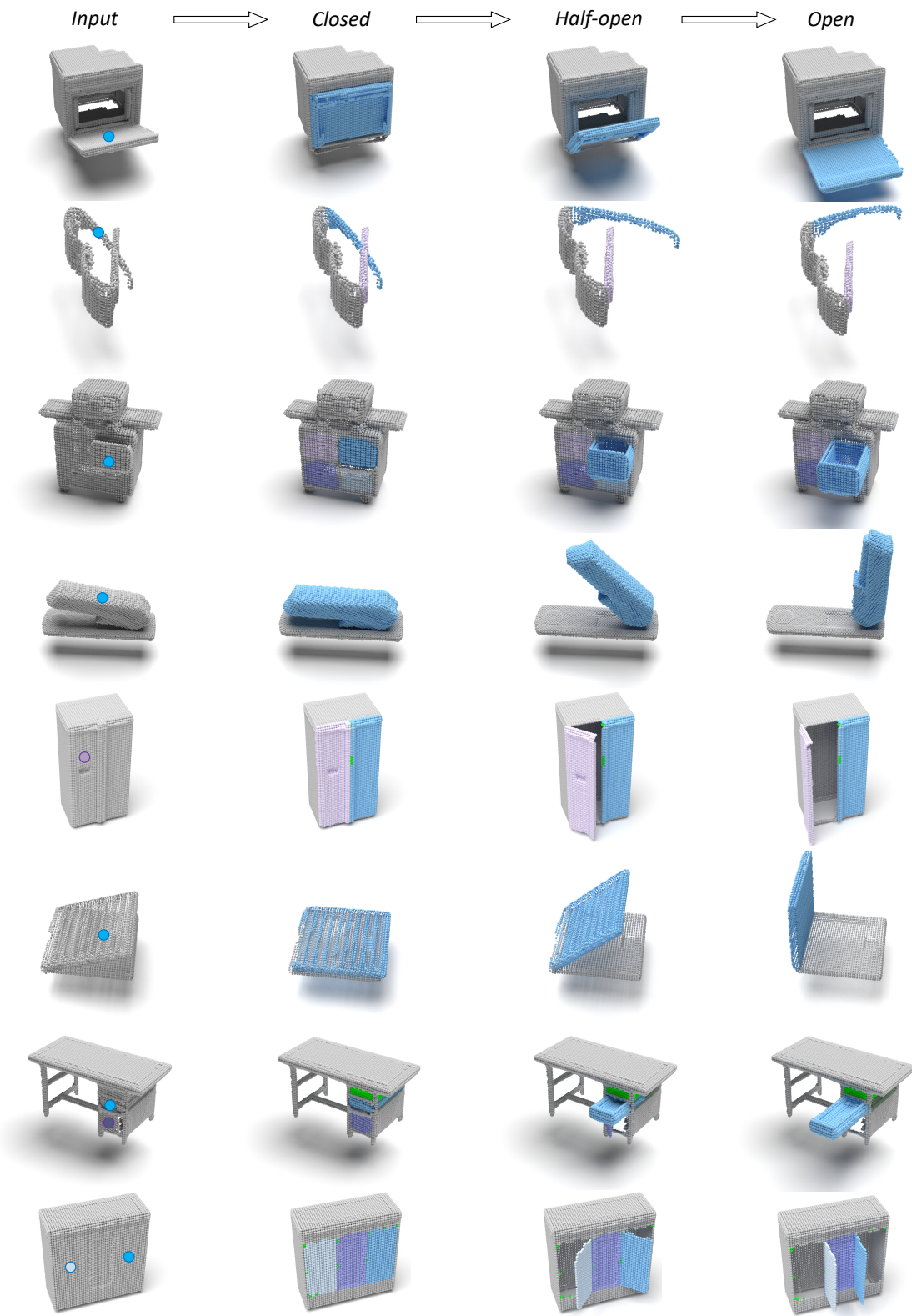
Figure 11. Visualizing how Cart enables object manipulations. Distinct object parts have different colors. The dots in the leftmost column denote the parts chosen to be operated.
