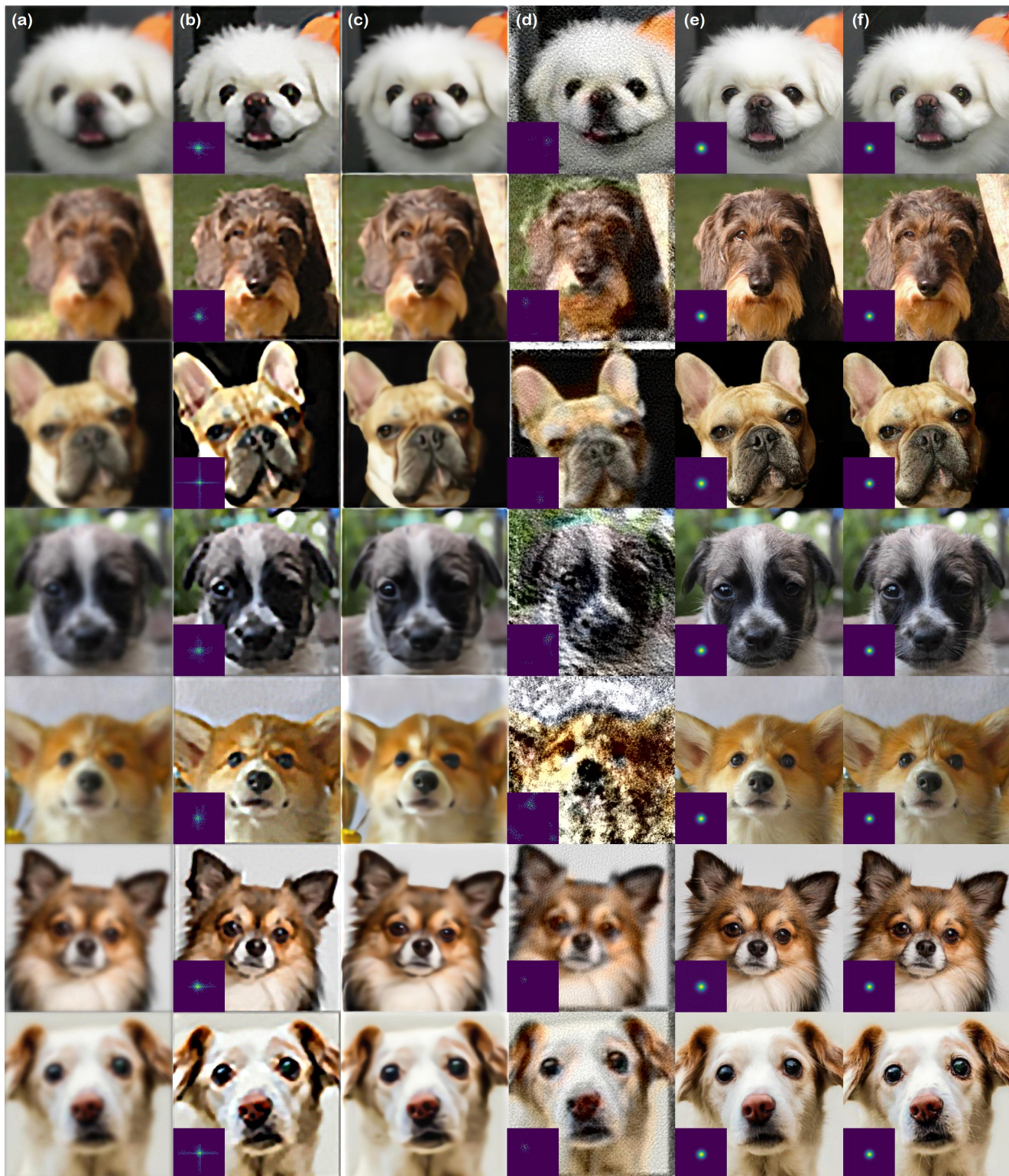
Figure G.4. Blind Gaussian deblurring results on the AFHQ 256 \times 256 dataset. (a) Measurement, (b) Pan-DCP [44], (c) MPRNet [61], (d) SelfDeblur [47], (e) BlindDPS (ours), (f) Ground truth.
