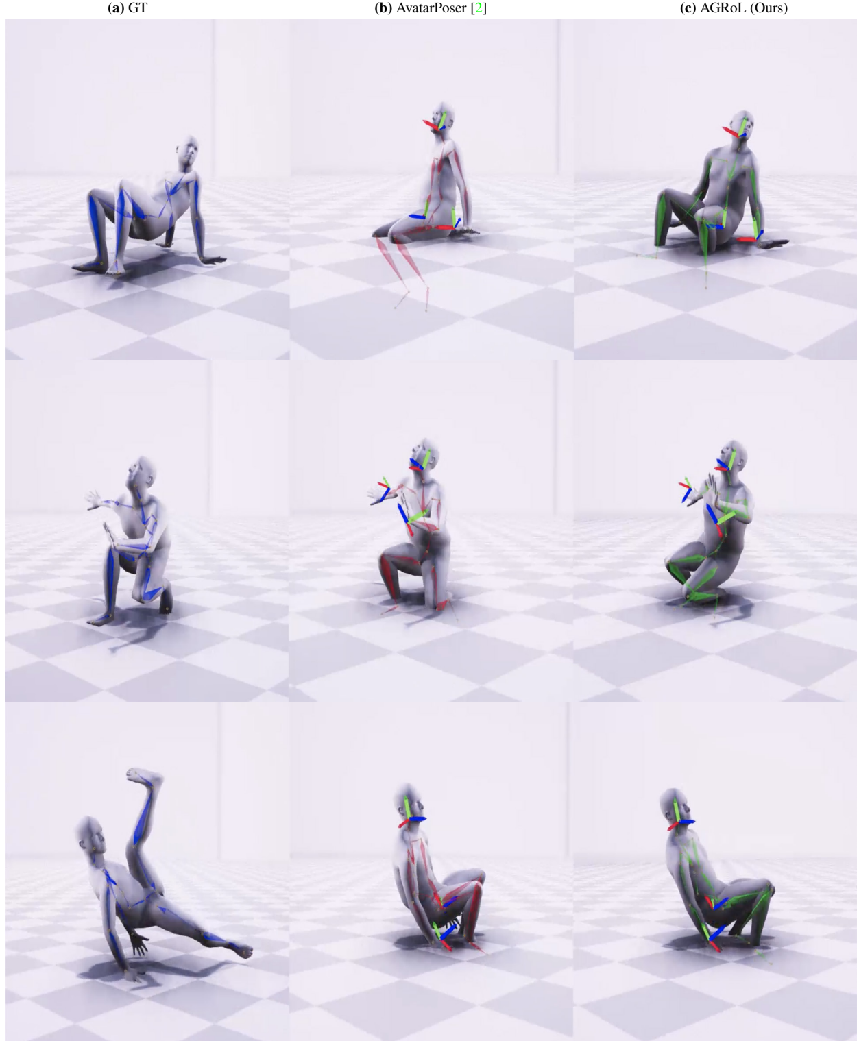
Figure II. Failure test cases. We visualize the predicted skeletons and human body meshes: (a) Ground truth skeletons in blue, (b) AvatarPoser predictions in red, (c) AGRoL predictions in green. The models were trained on the subset of AMASS [5] following the protocol of [2]. In the figures, the RGB axes indicate the position and orientation of the head and hands, which are used as input to the models. We can observe that our method struggles with (i) irregular poses that were not well-represented in the training set, resulting in inaccurate poses and floor penetration, and (ii) when the lower body pose is not strongly correlated with the upper body, as seen in the break dance motion in the bottom row. To address these failure cases, we could consider increasing the diversity of training motions and incorporating additional physical constraints.
