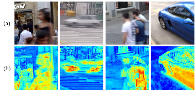
Figure 4. The visualization of the learned attention features in KAM. (a) The blurry image. (b) The learned attention features.
