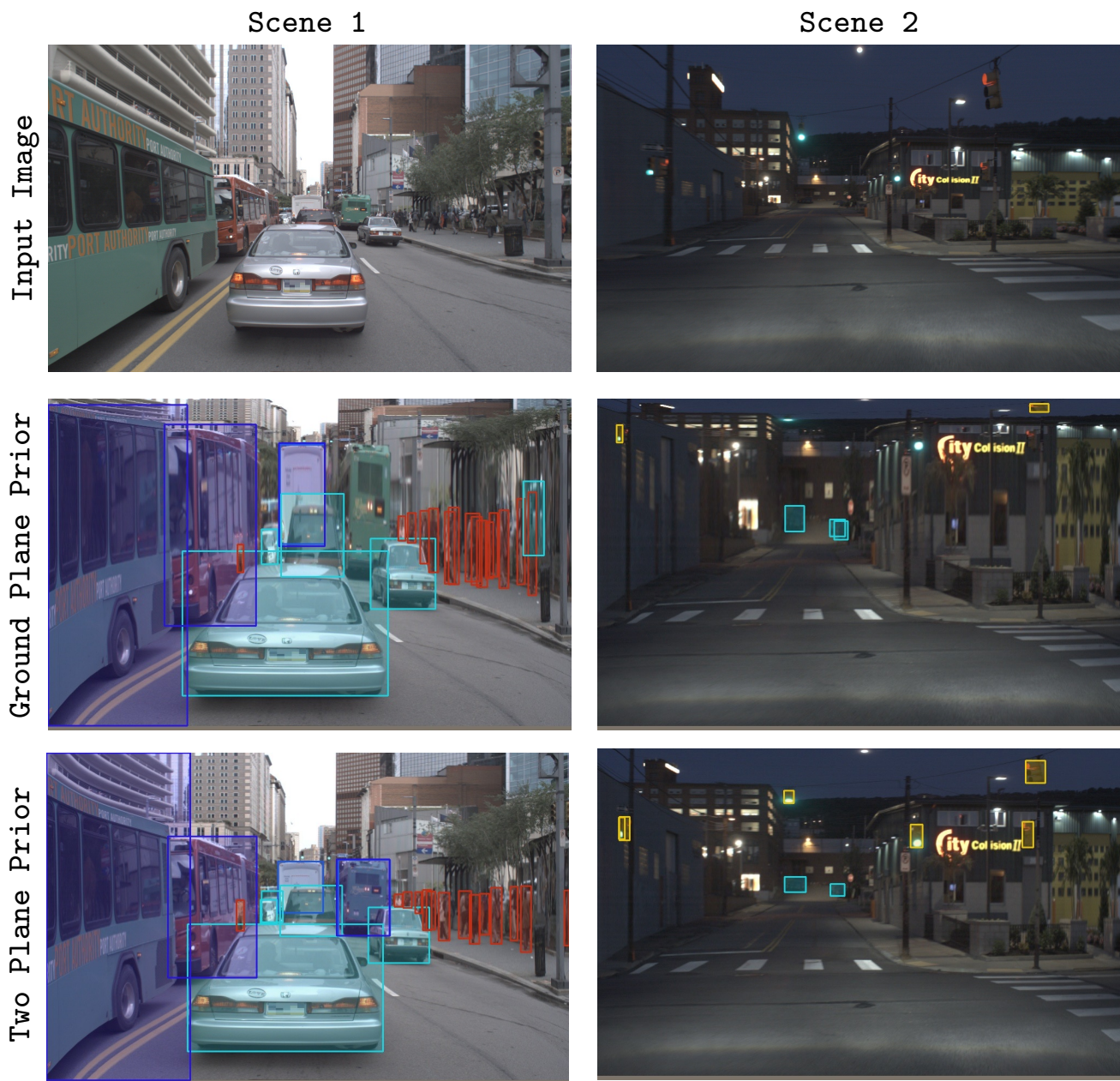
Figure 5. Ground Plane Prior vs Two-Plane Prior: This figure demonstrates how crucial it is to model the second plane. Learning is difficult with Ground Plane Prior (Section 5.1 in the manuscript) and causes heavy distortion of non-ground-plane regions.
