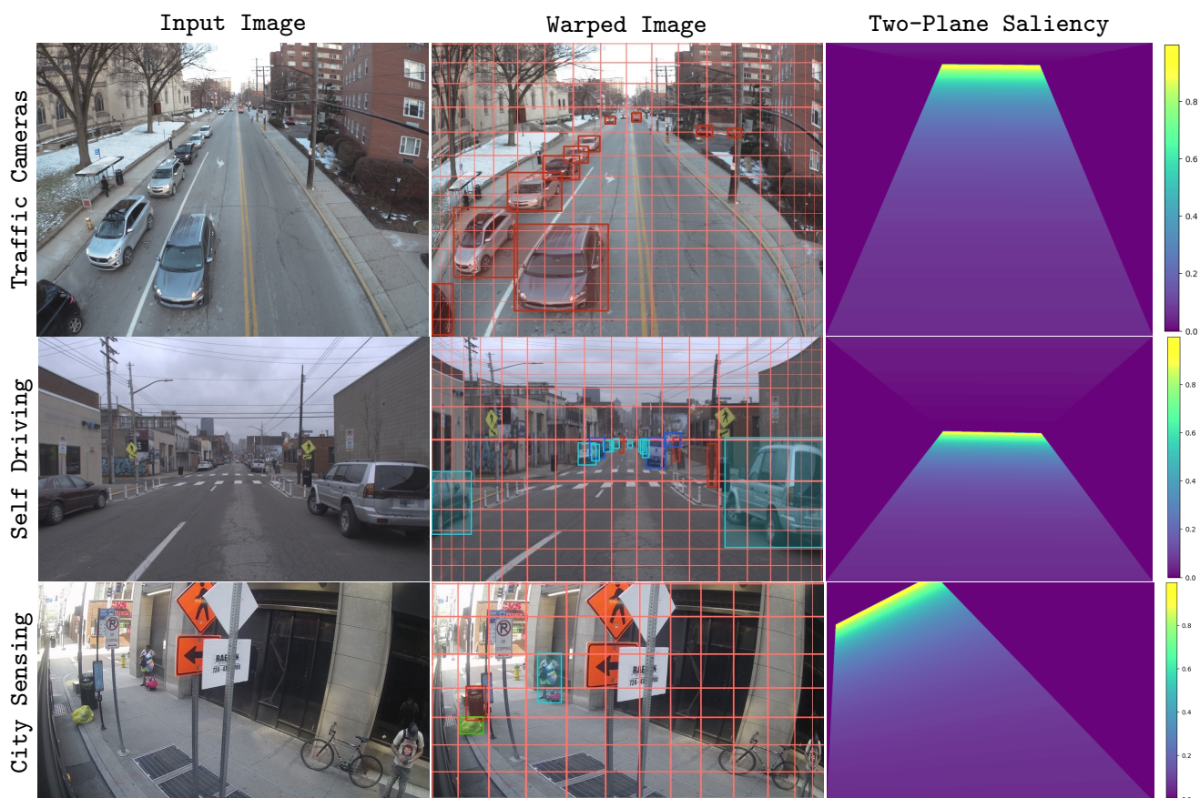
Figure 4. Two-Plane Prior Based Warping: Two-Plane Prior is defined by a few parameters that describe two planar regions in the direction of the vanishing point in the 3D scene (See Section 3.1 and 3.2 in manuscript). Firstly, we can observe the Two-Plane Prior’s explicit dependence on the vanishing point v in the saliency maps. Next, as we can observe from grid lines (equidistant in the original image) overlaid on top of the warped images, the extent of spatial warping varies across datasets (WALT, Argoverse-HD and Commuter Bus), showing us the need for learnable parameter \nu over prior work which do not directly model this relationship. Lastly, notice the second plane’s effect in sampling. The second plane acts as a “counter-balance” to reduce distortion, and the plane is faintly observable (contrast adjusted for better visibility).
