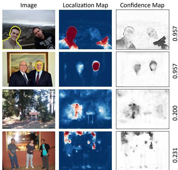
Figure 5. Examples of forged (top) and pristine (bottom) images (forgeries are highlighted in yellow). We show the localization map, the confidence map and the integrity score. For real images despite the anomaly map presenting some false alarms, the confidence analysis helps to make a correct prediction.
