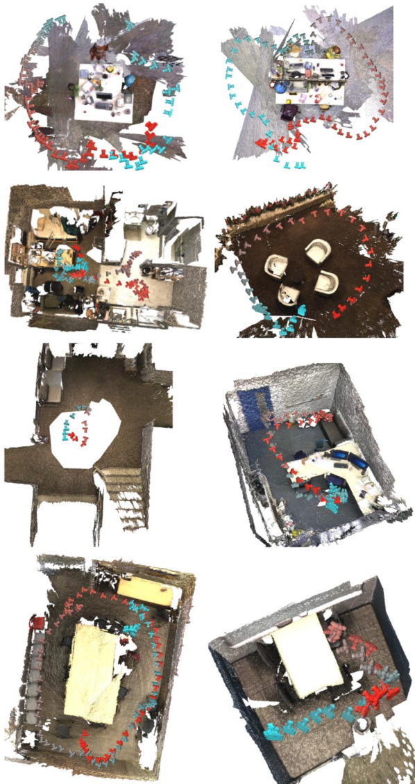
Figure 2. Example scene reconstructions from TUM RGB-D [22] and ScanNet [4] with optimized camera trajectories. Interpolation of camera color from blue to red represents the temporal order of cameras. Geometric reconstructions are obtained using scalable TSDF volume integration [3, 25].
