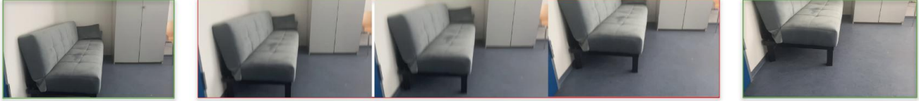
Figure 3. A self-captured sequence of frames with a smartphone. We show that two non-blurry frames on the left and right are apart by > 20 frames, where motion blur is measured using the variance-of-Laplacian thresholding. We show three sample frames in between that are affected by the motion blur. Hence, low FPS registration would have real-world use in scenarios where frames not affected by motion blur must be considered for registration.
