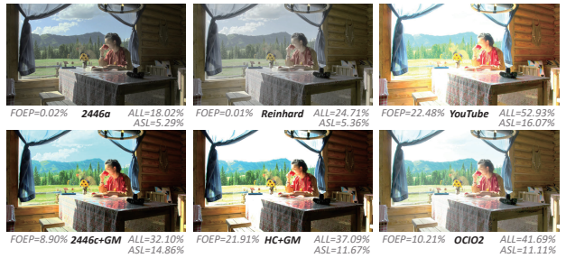
Figure 5. SDR images generated by different degradation models (DMs), from same HDR. As seen, tone-mapping operators (TMOs) like 2446a and Reinhard dedicate to preserve as much information from HDR, so their SDRs are of less FOEP (fraction of over-exposed pixels). Also, from ALL (average luminance level) and ASL (average saturation level) we now that current DMs in first row tend to exaggeratedly alter the style from HDR to SDR, so network will learn a vise-versa SDR-HDR style tendency which do not follow the technical and artistic intend of origin SDR.
