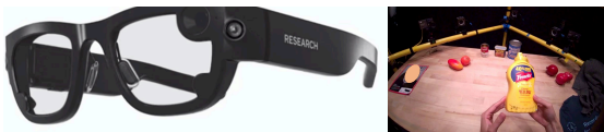
Figure 1. Aria glasses. Aria glasses [2] provide egocentric views of the environment using cameras mounted on the glasses.
