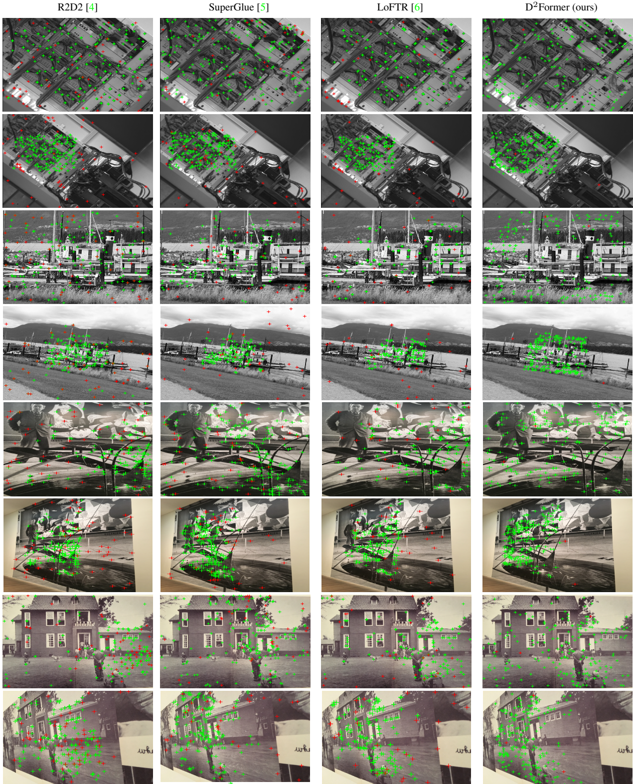
Figure 4. Qualitative comparisons under illumination variations on the HPatches. Green and red crosses denote correct and incorrect matches respectively (threshold is 3px). Our D 2 Former can extract discriminative feature description and realize robust keypoint detection under extreme viewpoint changes, leading to more accurate matching results.
