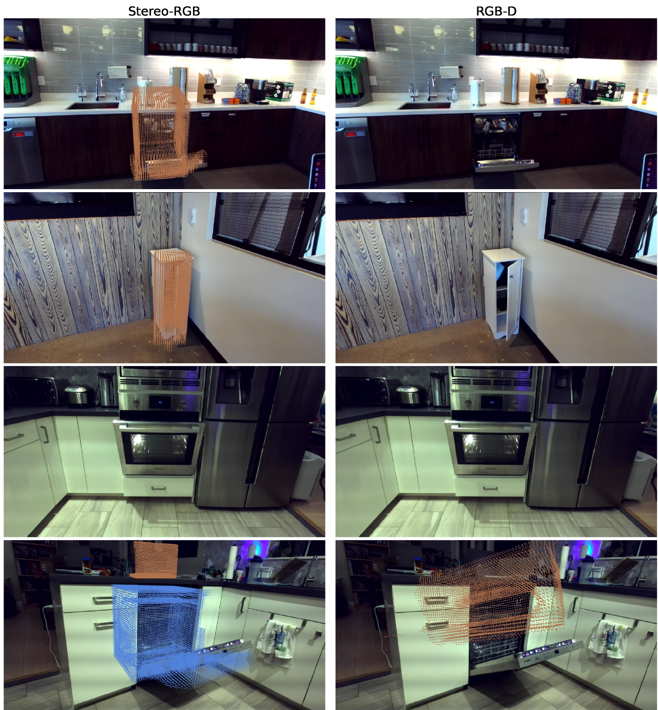
Figure S.8. Stereo-RGB Image (Left) vs. RGB-D Image (Right) Input. The first row shows a successful detection and reconstruction of CARTO in an office kitchen environment. Second row shows a reconstruction of a cabinet. Eventhough, CARTO has never seen objects from this category it highlight its generalization beyond the trained categories. The third and fourth row show two failure cases of either no detection at all (third row) or a misdetection of a laptop on the kitchen counter (fourth row). CARTO with RGB-D input is not able to reconstruct any objects.
