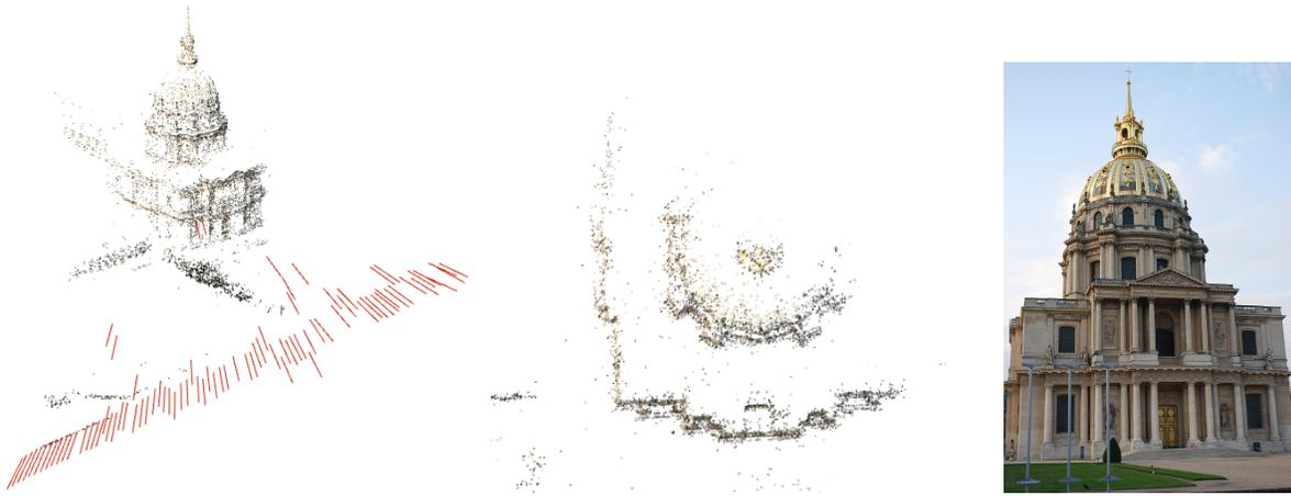
Figure 7. Qualitative results of 1D radial Structure-from-Motion on the *Eglise* dataset (85 images) from [62].
