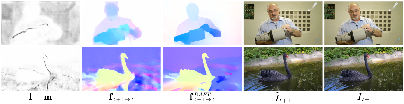
Figure 1: Visualization of the map 1 - \mathbf{m} , the optical flow \mathbf{f}_{t+1 \rightarrow t} , the optical flow by RAFT [4] \mathbf{f}_{t+1 \rightarrow t}^{RAFT} , the predicted frame \tilde{I}_{t+1} and the “ground truth” I_{t+1} .
