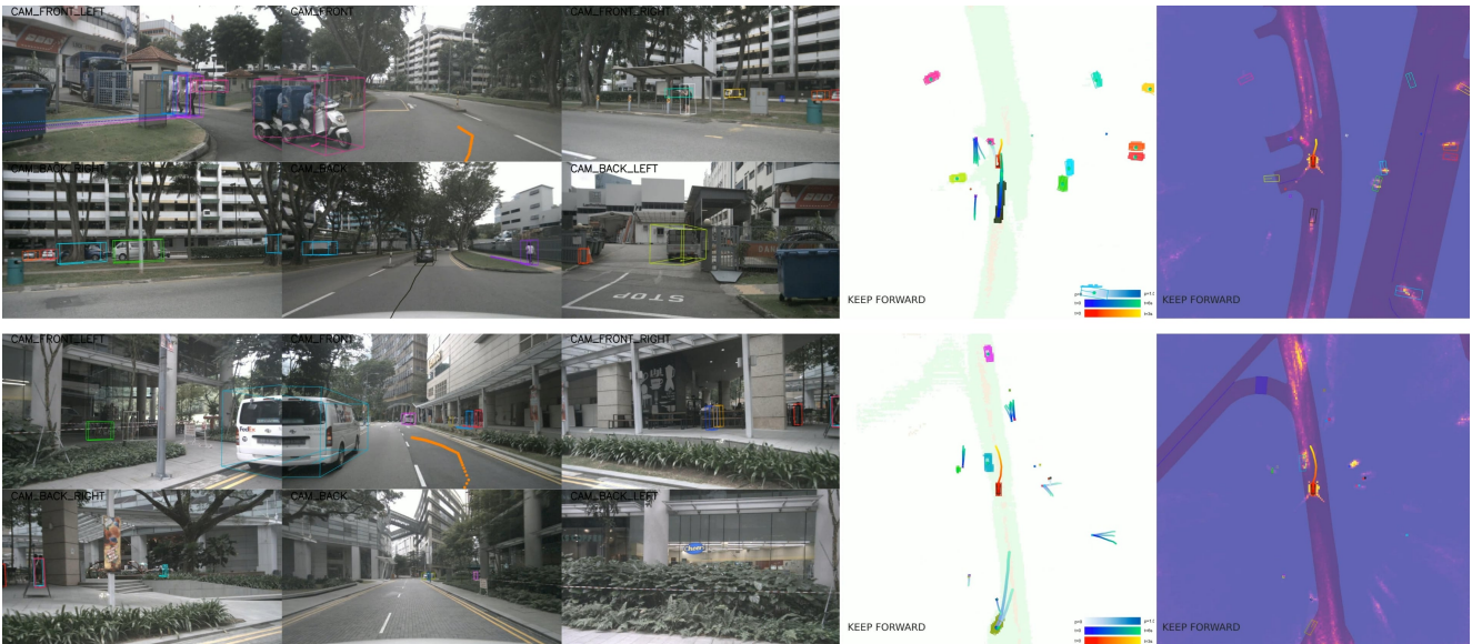
Figure 8. Obstacles avoidance visualization. In these two scenarios, the ego vehicle is changing lanes attentively to avoid the obstacle vehicle. From the attention mask, we can observe that our method focuses on the obstacles as well as the road in the front and back.
