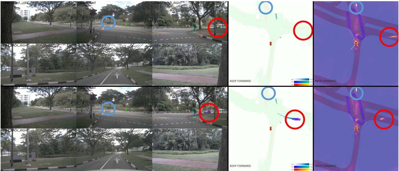
Figure 9. Visualization for planning recovering from perception failures. We show an interesting case where inaccurate results occur in prior modules while the later tasks could still recover. The top row and the down row represent two consecutive frames from the same scenario. The vehicle in the red circle is moving from a far distance toward the intersection at a high speed. It is observed that the tracking module misses it at first, then captures it at the latter frame. The blue circles show a stationary car yielding to the traffic, and it is missed in both frames. Interestingly, both vehicles show strong reactions to the attention masks of the planner, even though they are missed in the prior modules. It means that our planner still pays attention to those critical though missed agents, which is intractable in previous fragmented and non-unified driving systems, and demonstrates the robustness of UniAD.
