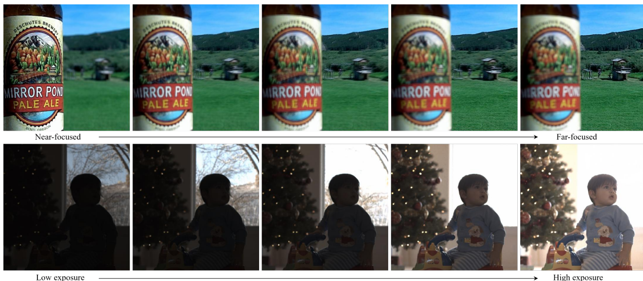
Figure 7. Controllable rendering results of our method. The leftmost and rightmost images are two training images, and the middle results are rendered with interpolated focus or exposure.
