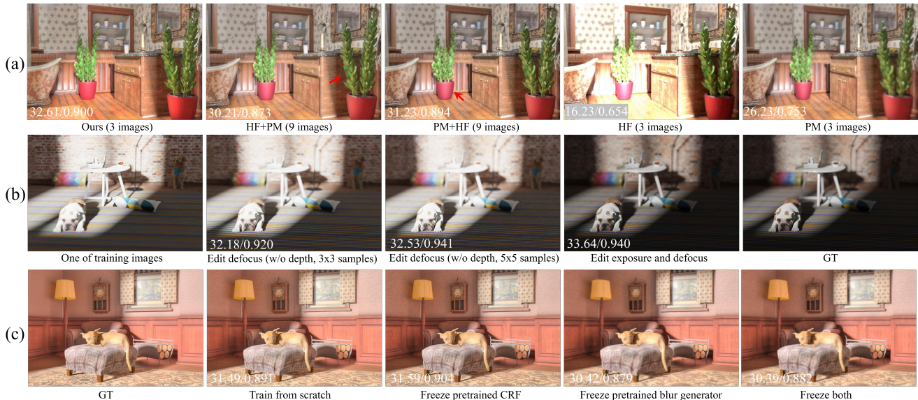
Figure 2. (a) Comparisons with two off-the-shelf optimization-based algorithms. “HF” is Helicon Focus software for all-in-focus images and “PM” is Photomatix software for HDR images. (b) Evaluations of our generated LDR and defocused images. (c) Evaluations on a new scene by freezing the pre-trained camera model. The first and third rows are all-in-focus HDR images. The PSNR and SSIM are presented in the lower left corner. Please open with PDF reader for zoom-in.
