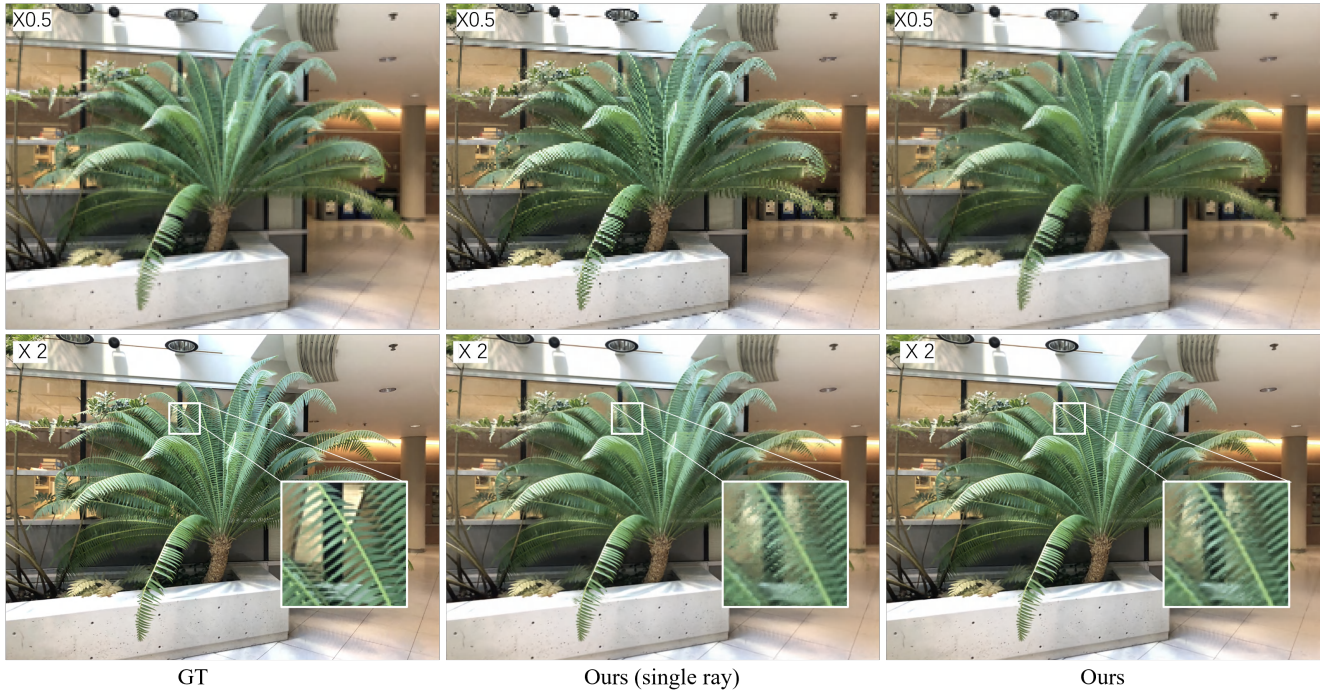
Figure S3. The qualitative results of our model that renders a pixel from a single ray. The top row shows the novel views rendered at \times 0.5 scale. Our model (single ray) produces aliased novel view. The bottom row shows the novel views rendered at \times 2 scale. Our model (single ray) produces novel view with artifacts at thin structures.
