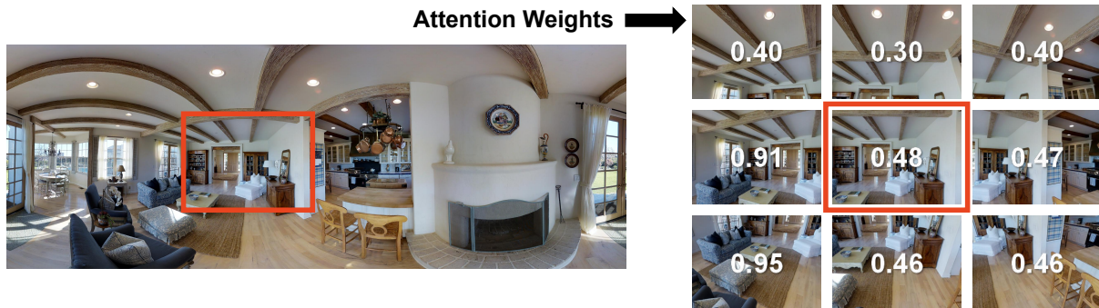
(a) The instruction is “Turn to your right and go pass the couch. Turn left and then turn right and stop by the couch”. According to the instruction “couch”, the two regions containing the sofa on the left side are given significantly more attention than the other regions.
