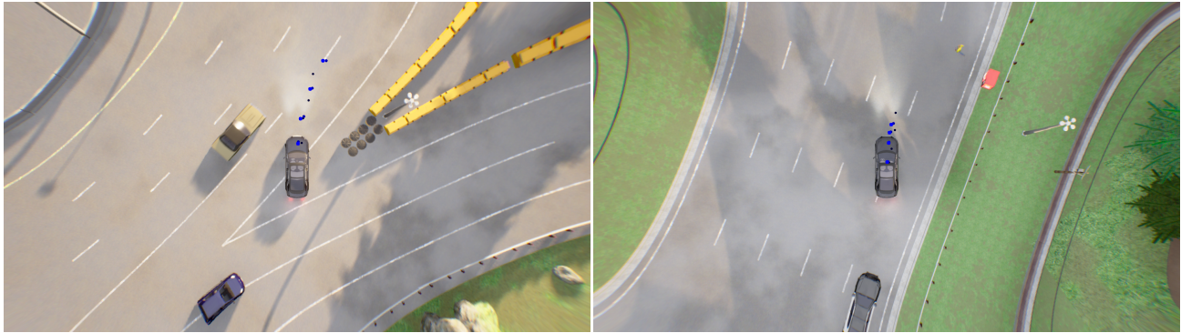
(c) Merge. The refined trajectory leaves more advance for the merging, which leads to a safer and smoother driving. (d) Lane Changing. The refined trajectory notices the jay-walker and leads to an emergency stop during the lane-changing process.
