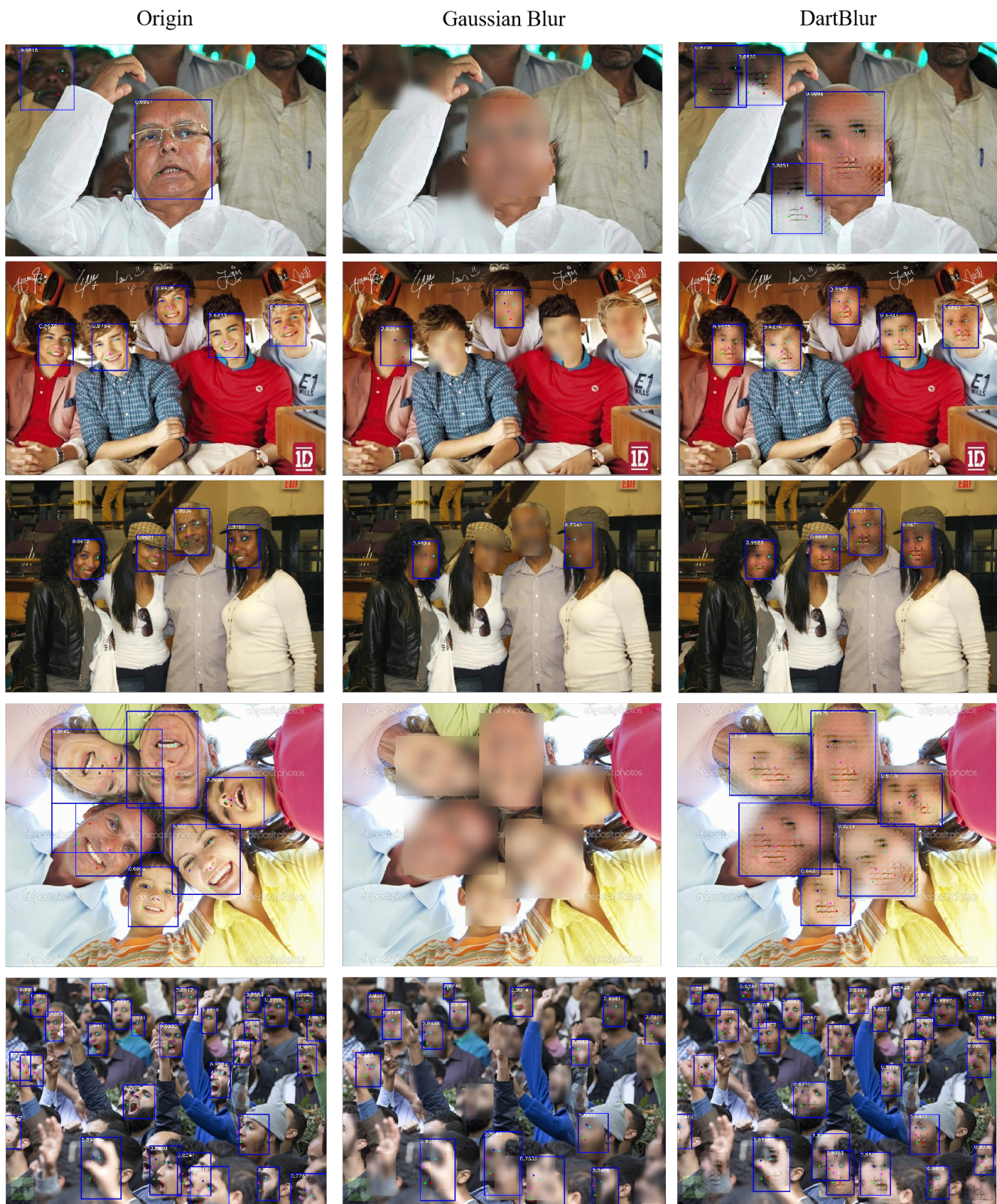
Figure 5. Comparison among detection results of “clean” RetinaFace on the WIDER FACE testing dataset. Left column: face bounding boxes detected on clean images. Middle column: detection results on Gaussian blurred images. Right column: detection results by on DartBlur images.
