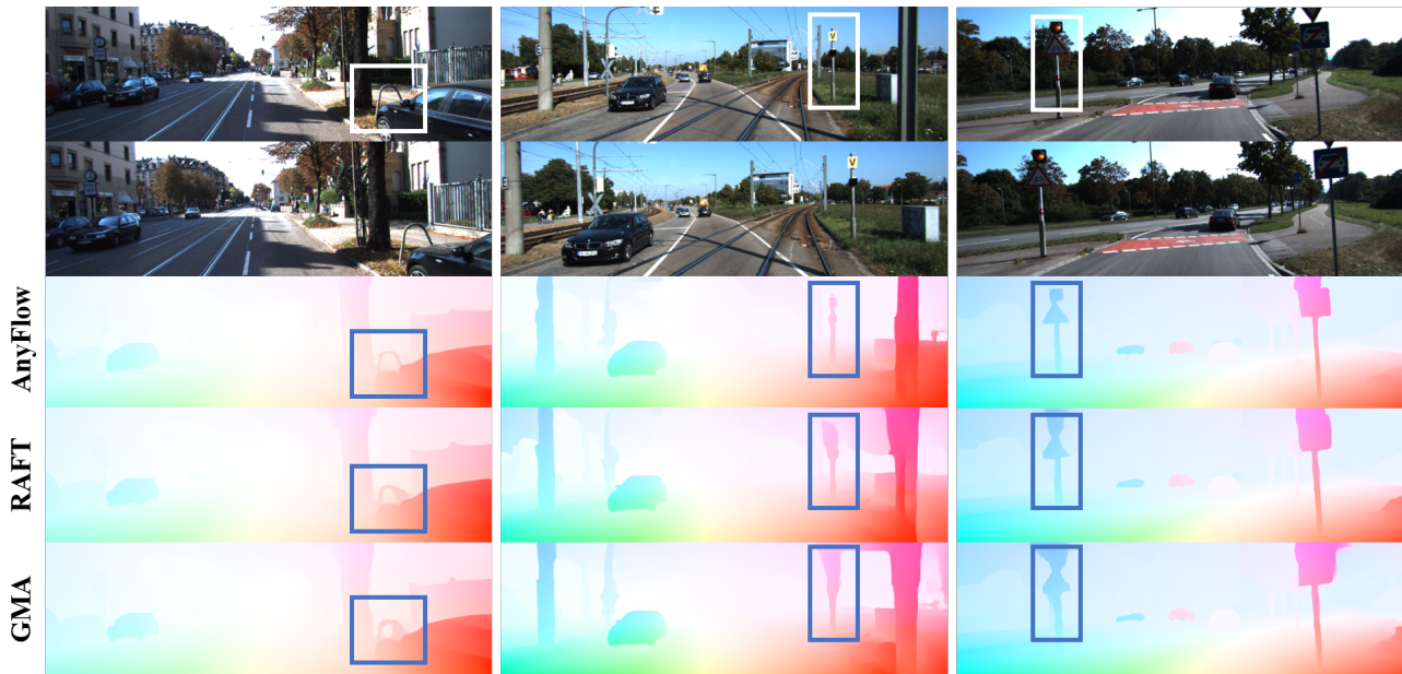
Figure 4. Qualitative results of AnyFlow, RAFT [9] and GMA [5] on KITTI test images. AnyFlow shows clearer and more accurate shape of objects with detail preservation.
