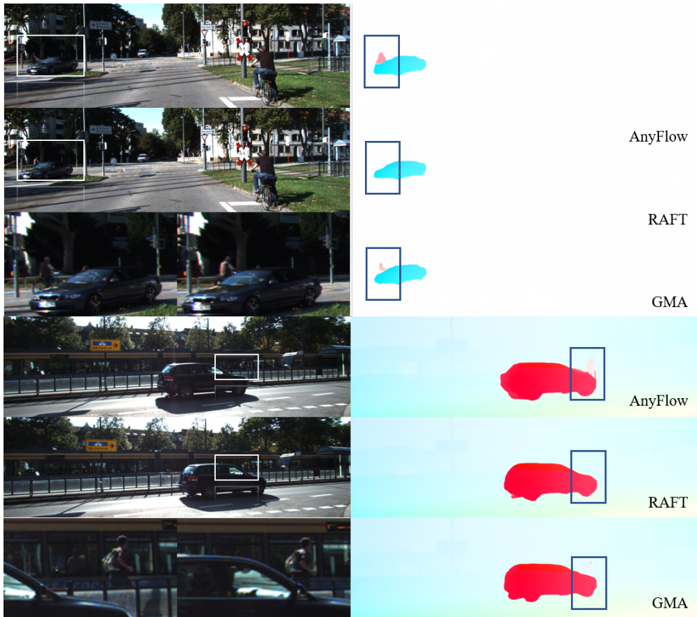
Figure 5. Qualitative results of AnyFlow, RAFT [9] and GMA [5] on KITTI test images. AnyFlow detects small objects and small motions well, where the other methods fail to detect.
