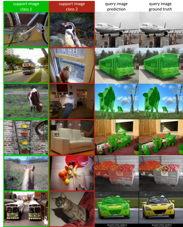
Figure 4. 2-way 1-shot segmentation prediction of CST trained with image-level labels. Image frames on the support images distinguish classes by colors.
