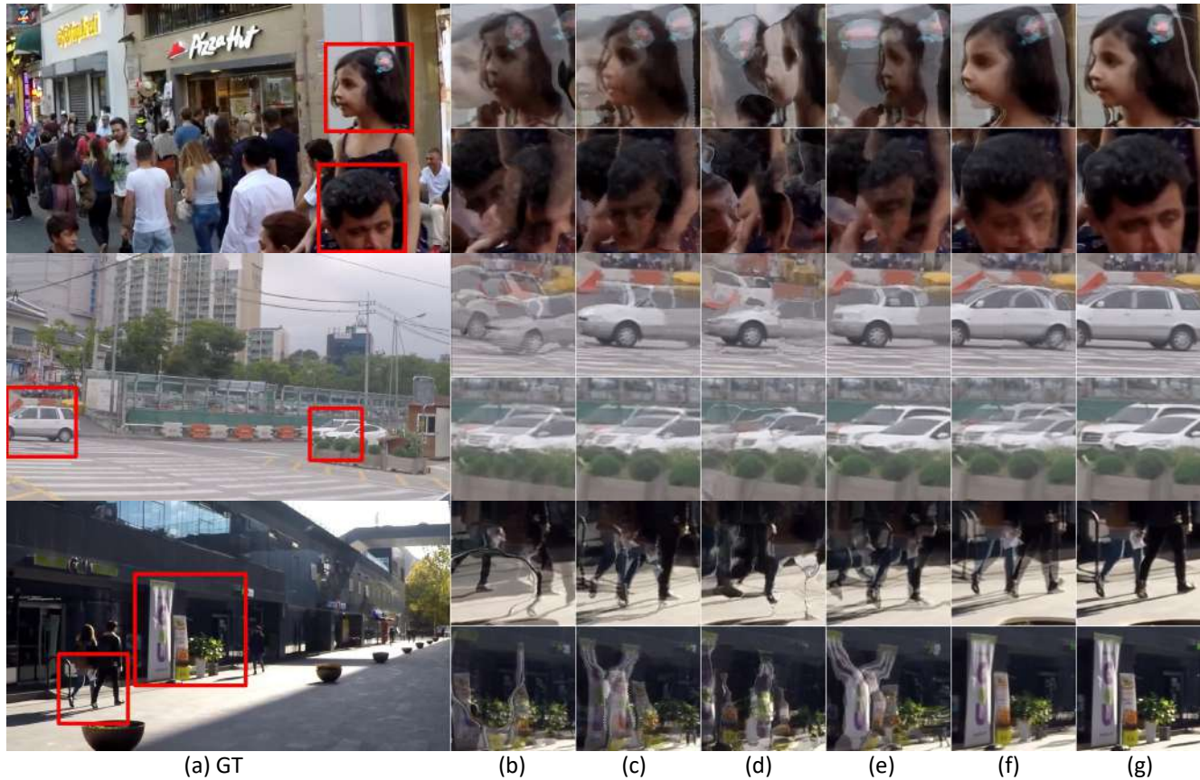
Figure 4. The qualitative comparison on the warped frame of estimated inter-frame motion fields on GoPro dataset. In order, (a) GT frame, (b) SuperSloMo [4] (c) BMBC [8] (d) ABME [9] (e) RIFE [3] (f) TimeLens [14] (g) Ours. As in the results, we confirm that our method produces more accurate warped frames than state-of-the-art inter-frame motion fields estimation methods. Please zoom for better visualization.
