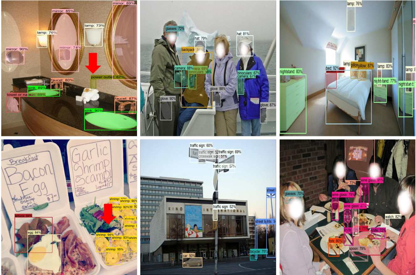
Figure 2. Objects365 transfer detection visualization (prediction) . Our trained RO-ViT is able to perform on a new dataset without any finetuning, and captures many challenging categories including novel categories (pointed by red arrows, e.g., power outlet and shrimp ).
