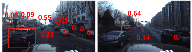
Figure S-4. Visualization of relation-aware attention scores. Red texts are relation-aware attention scores for a car in a red box to the other cars.
