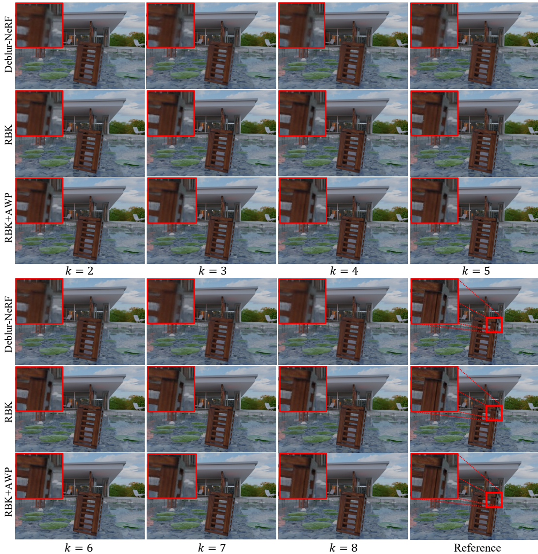
Figure 10. Qualitative results of ablation study depending on the number of rigid motion on camera motion blur scene. k denotes the number of rigid motion. Each row denotes Deblur-NeRF, DP-NeRF(RBK) and DP-NeRF(RBK+AWP), respectively. Red colored box in corner of images are enlarged part of same colored box region in reference images.
