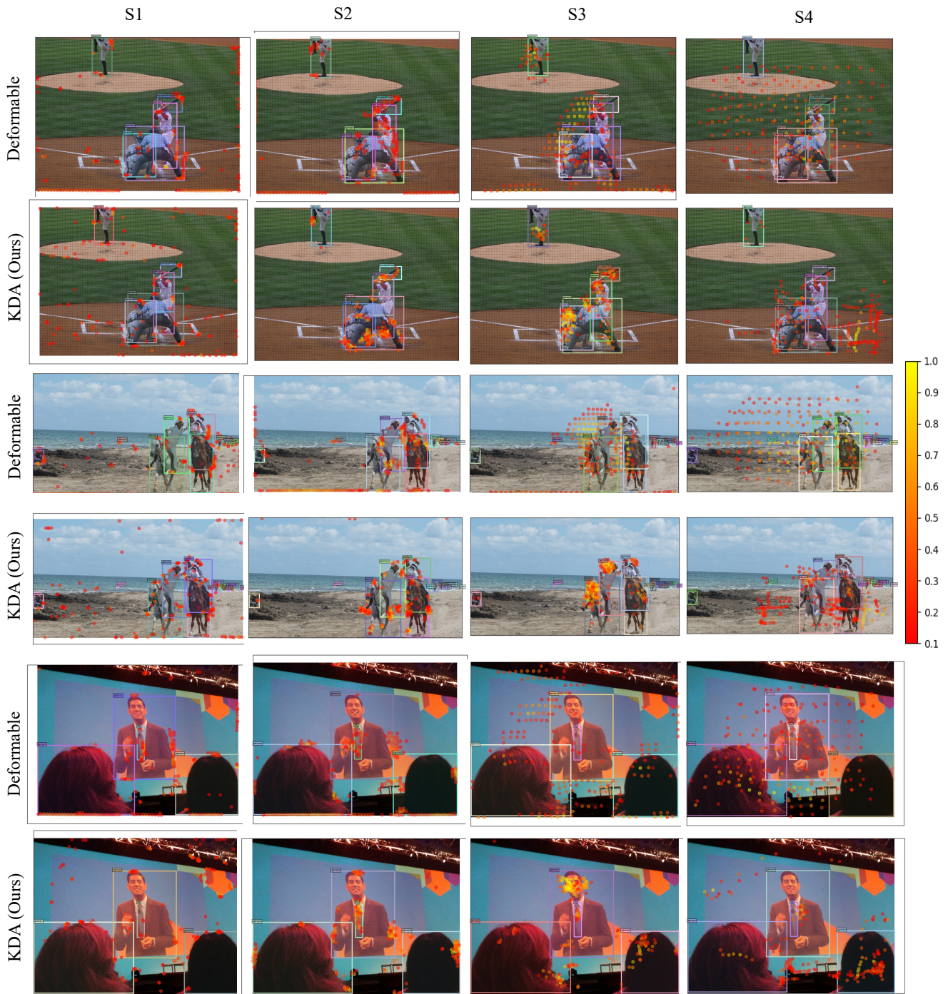
Figure 4. Visualization comparison of deformable and KDA attention in our Lite DINO from all feature scales. In high-level feature maps (S1, S2), KDA and deformable attention show similar attention regions. However, kDA can sample more meaningful locations on low-level maps (S3, S4), which indicates KDA can better extract local features from low-level maps and improve average precision in small object detection.
