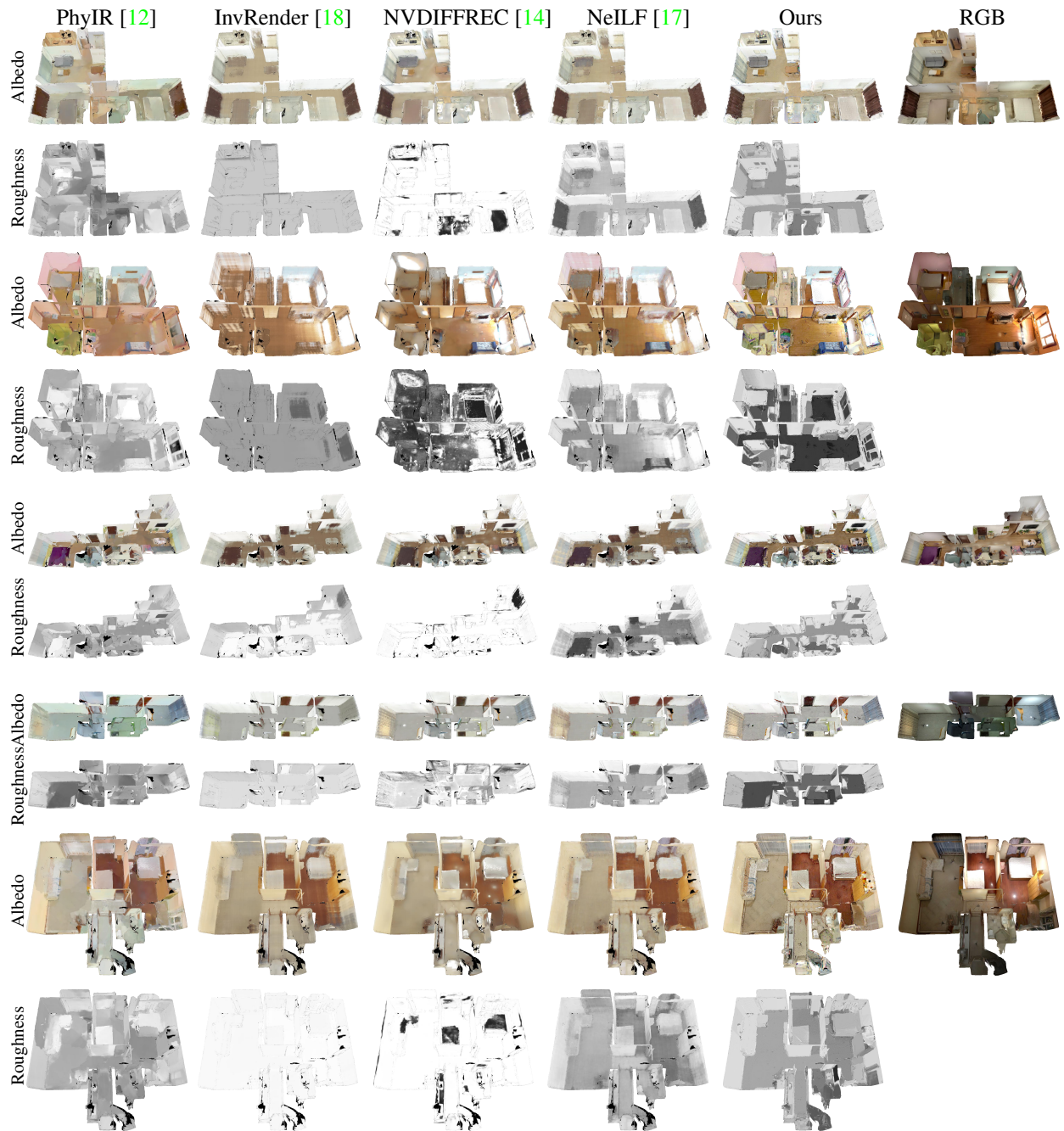
Figure 8. Additional samples of qualitative comparison in the 3D mesh view on challenging real dataset. From top to down: Scene 7, Scene 8, Scene 9 and Scene 11. Our method reconstructs globally-consistent and physically-reasonable SVBRDFs while other approaches struggle to produce inconsistent results and reduce ambiguity of materials.
