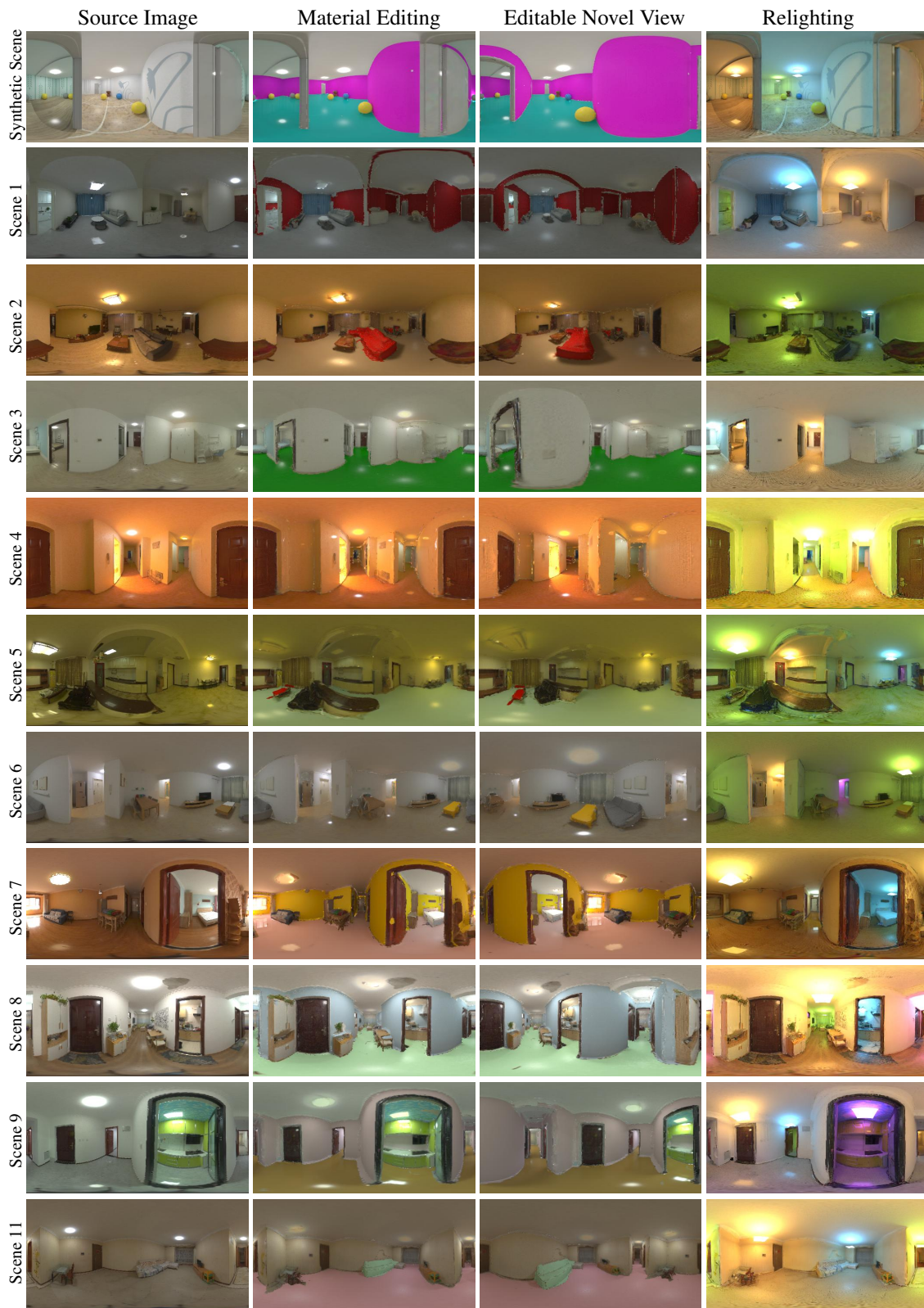
Figure 3. Additional samples of applications. We edit the roughness of floors in Scene 1, Scene 4 and Scene 6, and the albedo for all scenes. Compared to source images, our method still reproduces realistic and consistent lighting effects after editing.
