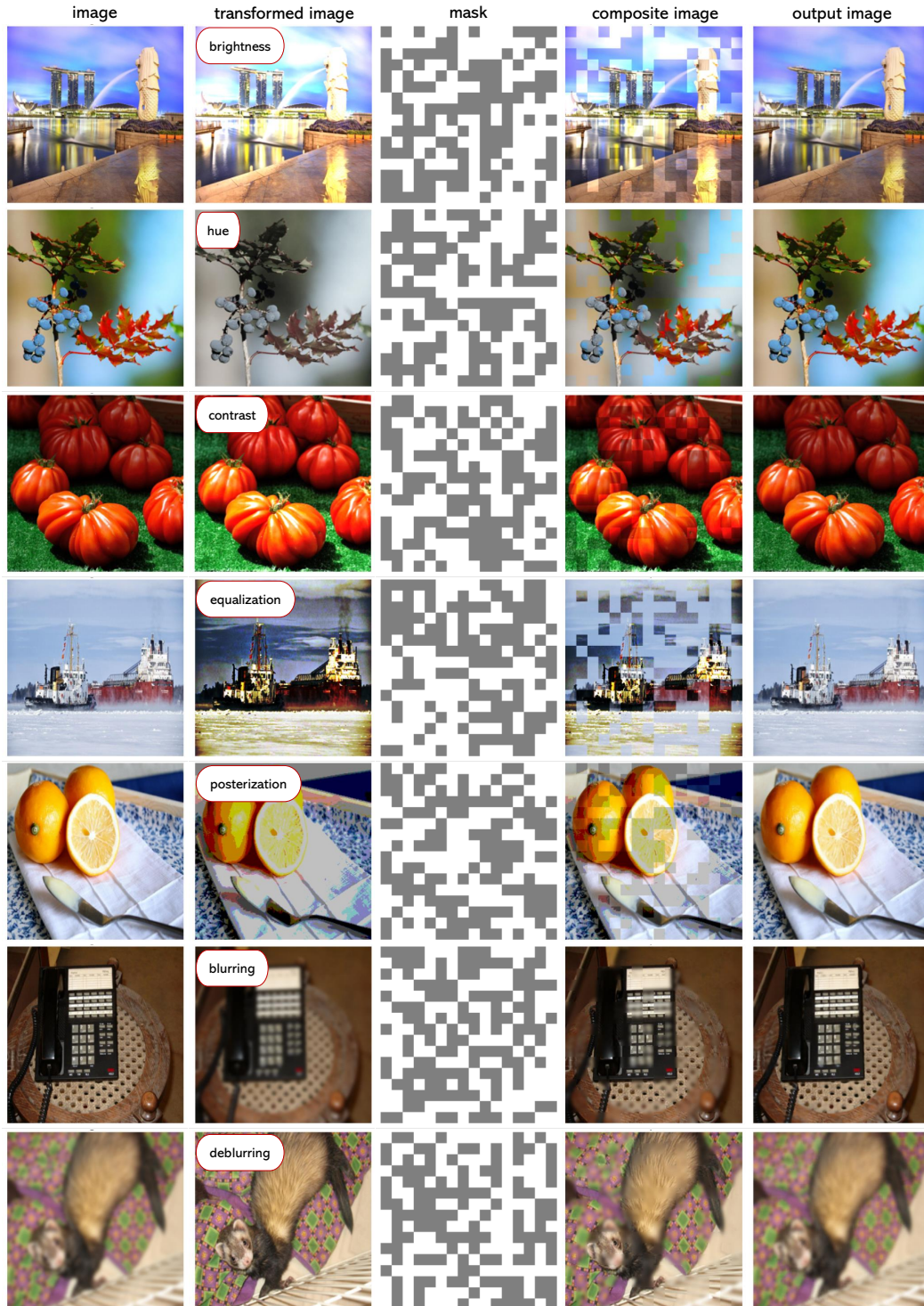
Figure 2. Qualitative examples that show data generated for pre-training and the output of a pre-trained LEMaRT model given the generated data. We apply brightness adjustment (row 1), hue adjustment (row 2), contrast adjustment (row 3), equalization (row 4), posterization (row 5), blurring (row 6), deblurring (row 7) to generate the transformed images shown in the second column.
