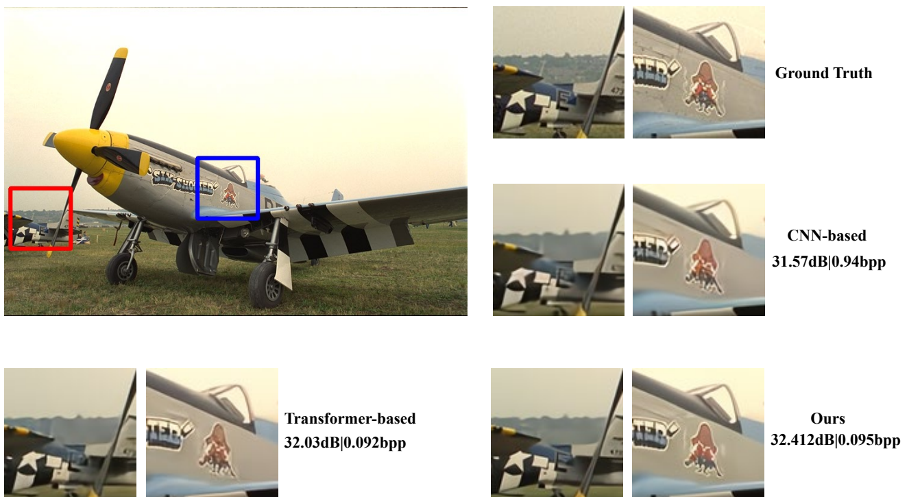
Figure 6. The visualization of kodim20 in Kodak dataset by using our TCM-based model, CNN-based model [4], and transformer-based model [11]. PSNR|Bit-rate is listed on the subfigures' right.
