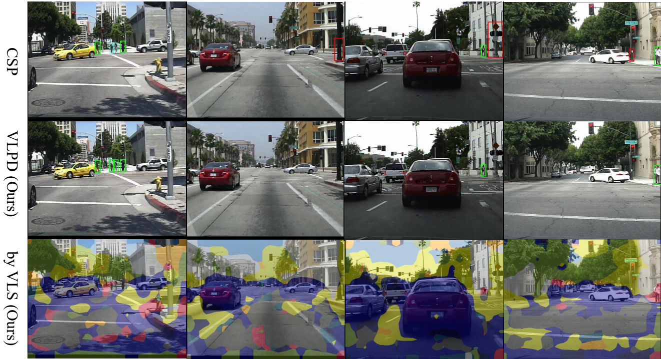
Figure 8. Qualitative analysis on Caltech [3] between our proposed VLPD and the baseline CSP [4]. Green bounding boxes are correct detections, red are wrong detections, and dashed blue are missing detections. Semantic classes of explicit contexts are obtained from our proposed VLS and colored following [1], e.g., “human” is red, “traffic sign” is yellow and “car” is blue.
