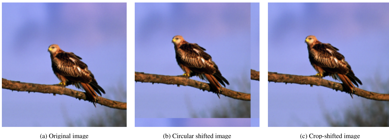
Figure 8. Visualization of used attacks. (a) Original ImageNet [6] validation-set image — 224 \times 224 center crop of the original 256 \times 256 image. (b): Circular shift of 16 pixels in x and y axes. (c): “Crop-shift” of the original image of 16 pixels in x and y axes; the cropped area is shifted, modeling moving the camera with respect to the scene in the bottom-right direction. The top-left part of the circular shifted and crop-shifted images are equal to the bottom-right part of the original image. The bottom and right edges of the circular shifted image consist of the top and left edges of the original image, causing unrealistic artifacts, while in the crop-shifted change we change the information from the scene.
