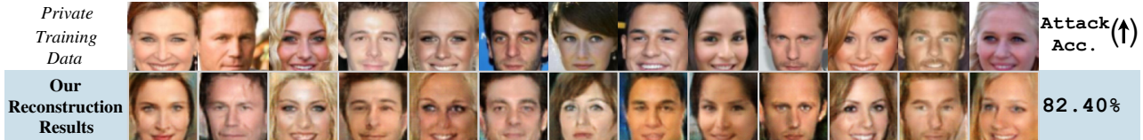
Figure 7. We show private data (top), our reconstruction results (bottom) and Attack accuracy ( \mathcal{D}_{priv} = \text{CelebA} [14], \mathcal{D}_{pub} = \text{CelebA} [14], M_t = \text{IR152} [8], Evaluation Model = face.evoLve [2], Inversion iterations = 2400) using GMI [20]. We remark that these results are obtained by combining L_{id}^{logit} and L_{id}^{aug} (referred to as + LOMMA throughout the paper).
