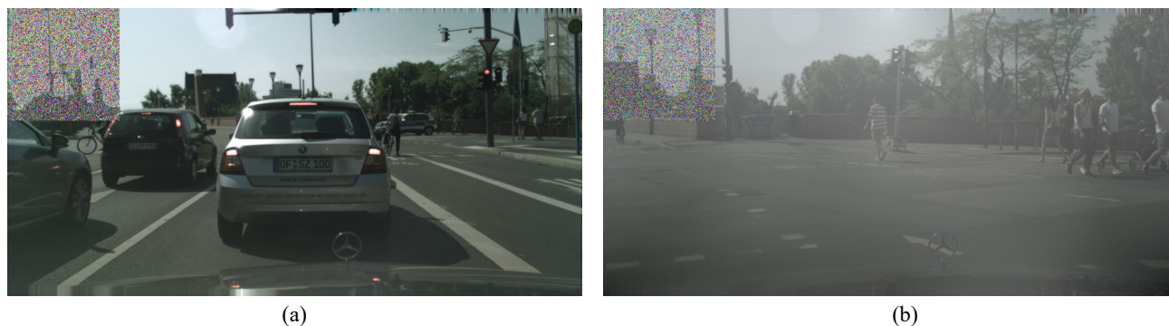
Figure 1. Visualization of the visual prompts. The visual prompt is added to the corner of the image, which pulls the distributions of the upcoming data closer to the training data’s distribution.
