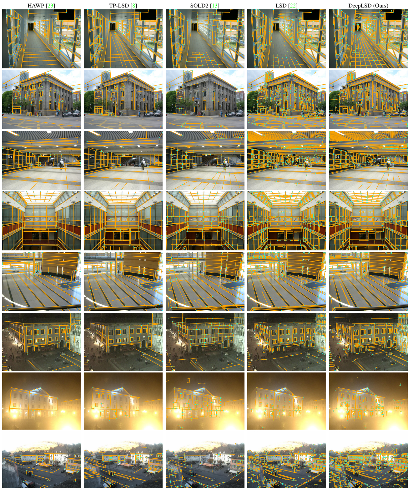
Figure 6. Visual comparison of line detectors. First five rows: the lines of DeepLSD (here, without line refinement) are more complete and accurate in urban scenarios (images from the YorkUrbanDB dataset [4]). Last three rows: when employed in challenging scenarios such as by night, over-exposition and low image quality, DeepLSD can detect more relevant lines than the other baselines (images from the Day-Night Image Matching (DNIM) dataset [25]).
