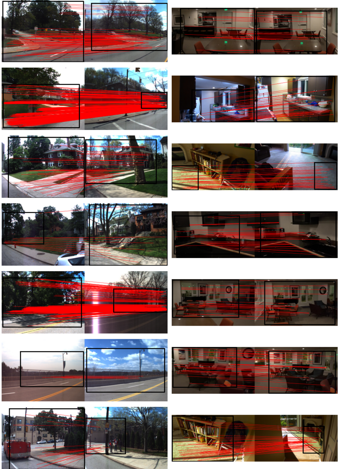
Figure A.1. Example pairs of images, along with 2D-2D correspondences between them, from the dataset used to train our approach.
