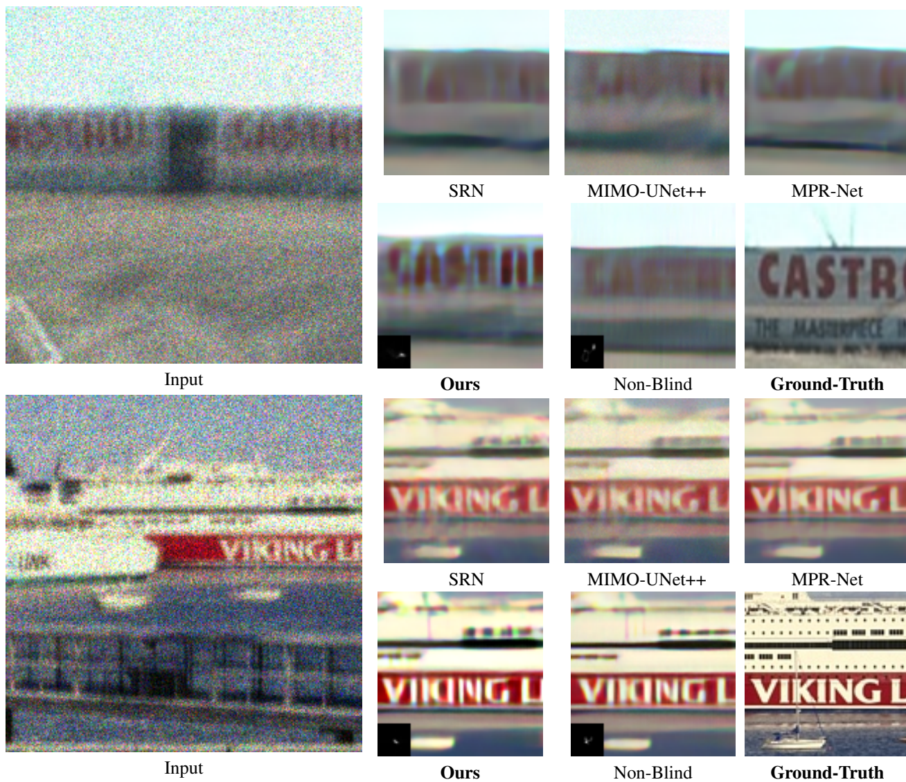
Figure 4. Qualitative Examples on Synthetic Blur: "Non-Blind" is provided for reference and serves as an upper bound on the deconvolution performance. It is obtained through PhD-Net with noisy-blurred image and ground truth kernel as inputs. The kernels in inset of "Ours" and "Non-Blind" represent the estimated and true blur kernel respectively.
