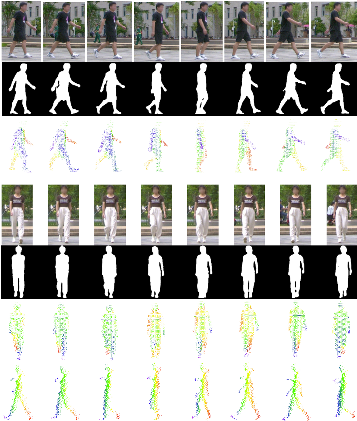
Figure 12. Exemplar sequences of SUSTech1K dataset under normal conditions. Eight frames in three modalities are visualized. The top three rows show three gait representations in RGB images, silhouettes, and point clouds. The bottom four rows represent gait representations in RGB images, silhouettes, front-view point clouds, and side-view point clouds. It shows LiDAR provides informative 3D geometry. (Best viewed in color.)
